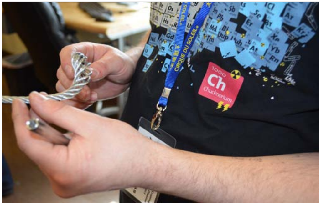
The sad results of destructive testing at Silver State Wire Rope
