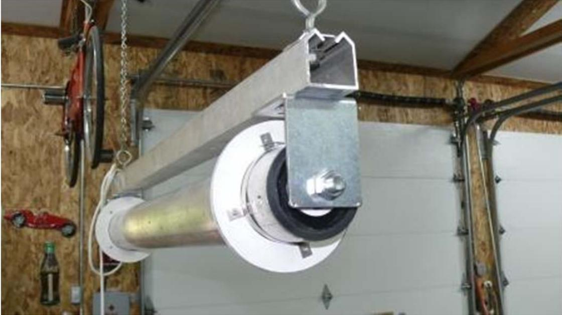
Flanges were installed on the drum to keep the fabric from spooling off the ends. Flanges are adjustable to the width of the soft goods.
