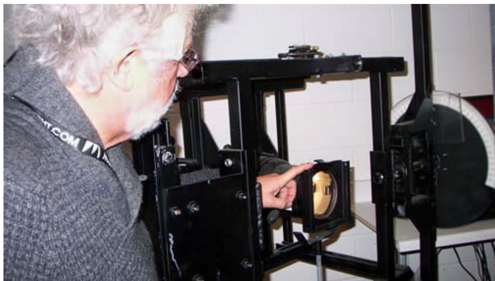
Rob Shakespeare, Professor of Lighting Design, demonstrates instrument alignment within the goniophotometer.
