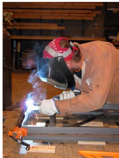
BFA senior Doug Dion welds the truss.
